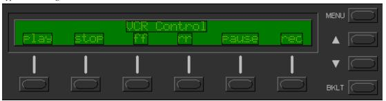
To give the user a visual cue that a function button has been pressed, it is possible to program active text. Double click on the object to display the "Edit Panel Object" window. Select a *Digital Channel* (join number) and enter *Active Text*. Click **OK**.
