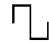
Figure 6: Square waveform of the signal used for calibration of the vertical scale.
