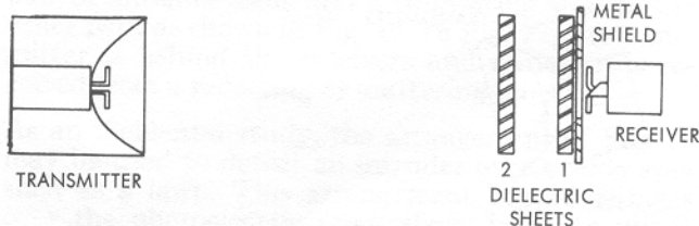
Fig. 21 Arrangement for Studying Interference of Microwaves Caused by a Thin Film of Air between Two Dielectrics
