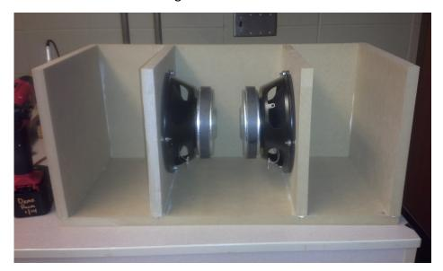
Assemble box—Drill two clear holes in the bottom panel along the rear edge. Good dimensions are 3/8" in from the rear edge and about 1" in. Align back panel and mark hole locations, then drill pilot holes. Fasten back panel on top of bottom panel with a THIN bead of construction adhesive and screw together. Make sure the back is flush with the rear edge of the bottom panel.
